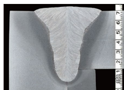
High heat input SAW (80mm) NSH-60S / Y-DL (One pass)
