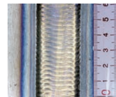
NITTETSU FILLER 196 in vertical up position
