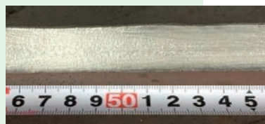
NF-800R of SAW-flux Fillet welding in Flat position
