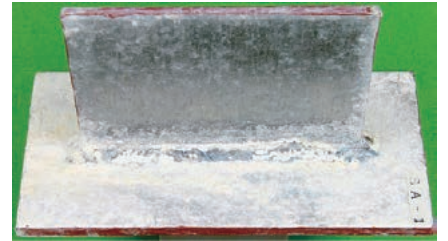
Prevent the rust in a 1000-hour saltwater spray test
