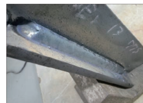
Photo.1 Example of vertical-up fillet welding, SF-3E (200A-13cpm, without weaving)
