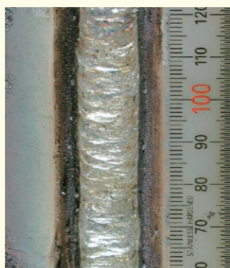
YAWATA™ WELD B (M) Vertical up
